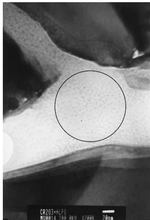
Fig. 5 AEM image from the aluminum phosphate sealant in between the lamellae. The ring in the sealant indicates the selected area for electron diffraction.
